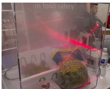
Figure 1. Photograph of 18''x18''x18'' fresh produce fogging chamber with open and packaged whole strawberries and spinach being treated (the lasers are used to visualize the flow of plasma-treated water microdroplets).
