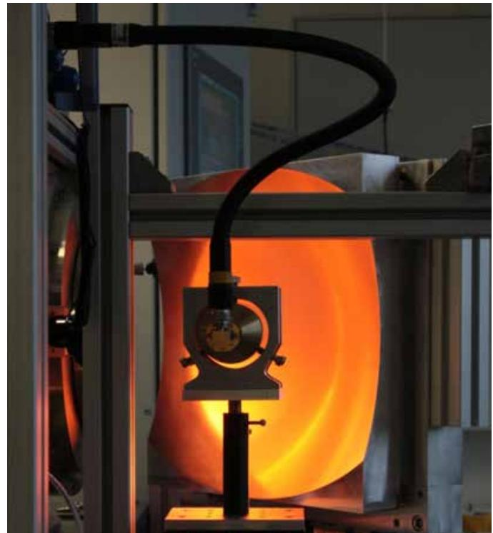
Electron density measurement with a 50 GHz interferometer at a low-pressure plasma discharge
