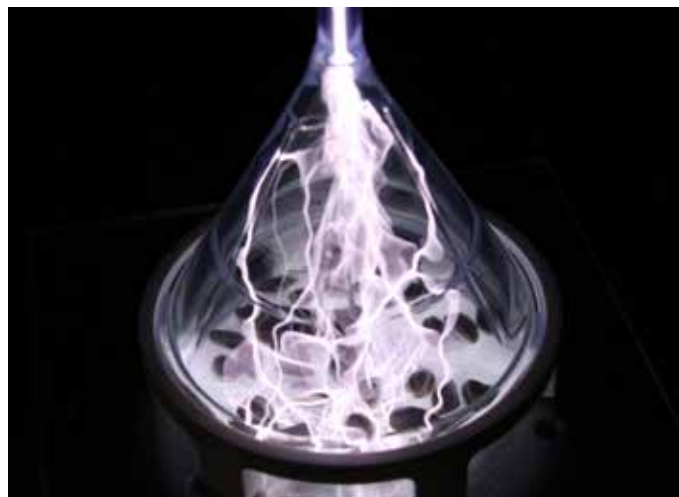
Treatment of sunflower seeds by corona discharge. The treatment kills micro-organisms on the surface of the grains. In addition, their ability to absorb water increases, and metabolic processes are stimulated.
