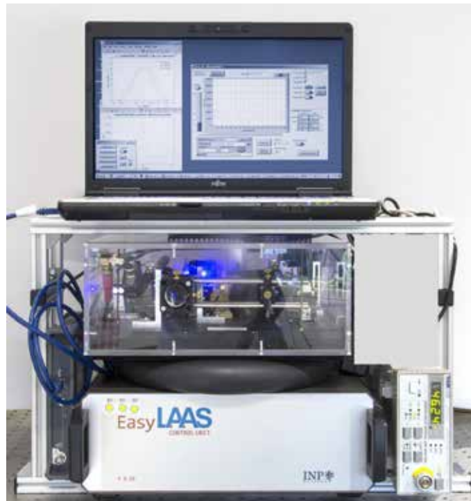
EasyLAAS system for laser absorption measurements
