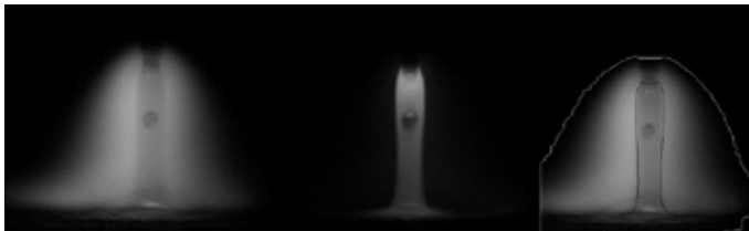
Synchronous recording of the arc (left image) with filters in the area of argon lines (left) and in the area of iron lines (right) as well as example of an image analysis (right image).
