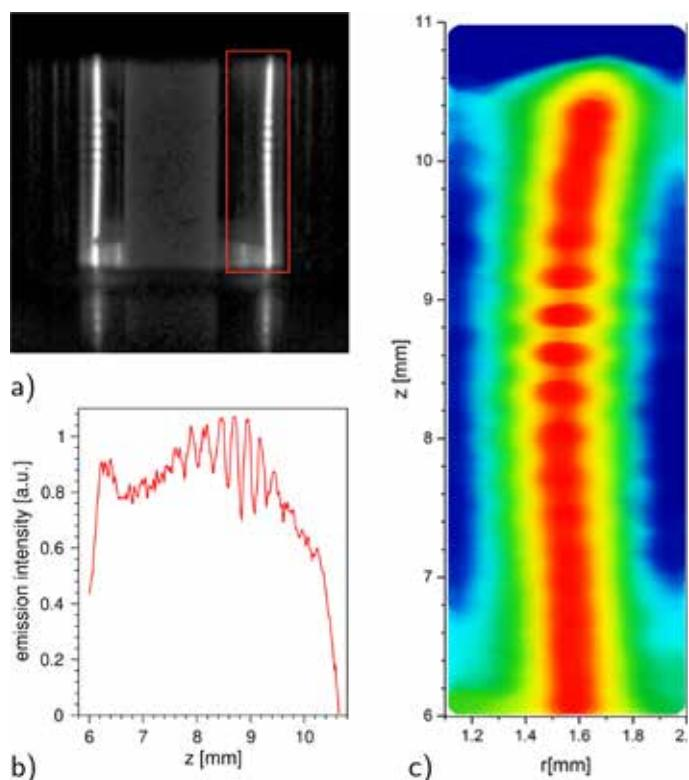
Atmospheric-pressure plasma: Structured discharge filament (striations) in experiment (a) and in the fluid model (b,c) (Sigenerger et al., Plasma Sources Sci. Technol. 28 (2019) 055004)
