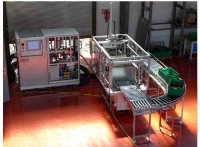
Process plant for treating products in Reusable Plastic Containers (RPC)
