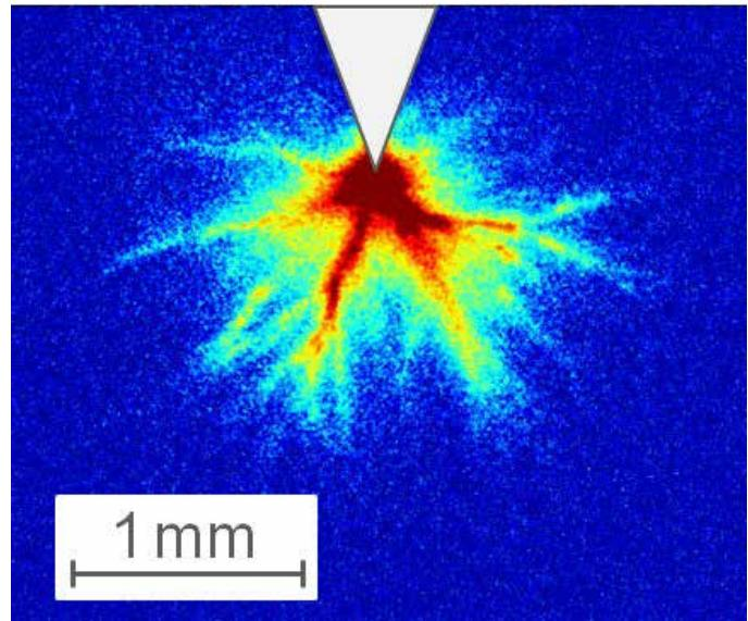
Reillumination (3 ns recording time) of a corona discharge ignited in water on the 20 ns falling edge of an applied high voltage pulse of 100 ns (FWHM) and 50 kV amplitude. For rapid decay, all channels of the original discharge light up again and suggest an appropriate current distribution.
