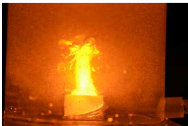
Microwave plasma (2.45 GHz) in water at atmospheric pressure
