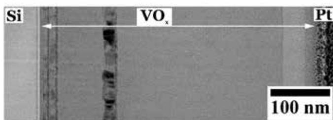
Vanadium oxide: Battery material of the future, film cross section:
