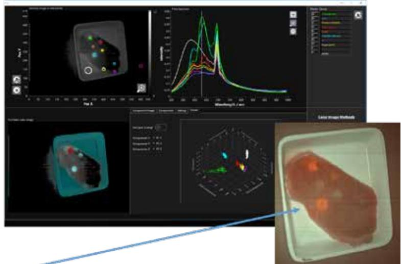
Recording spectra 24h after decontamination with micro organisms; infected spots are marked for each MO
