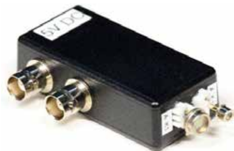
Completed sensor board equipped with 2 diodes. The compact size already achieved in the prototype allows easy installation in a safety helmet and can enable a much more compact size for mass production without the BNC measurement connections.
