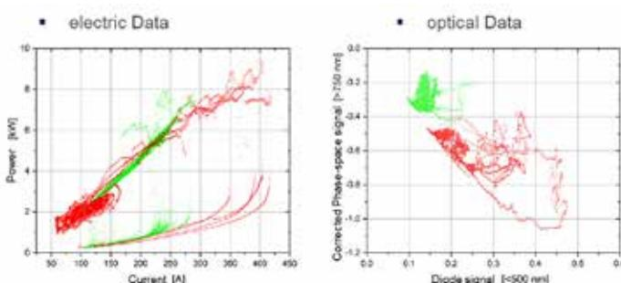
Red: faulty process part, green: non-faulty process part.
