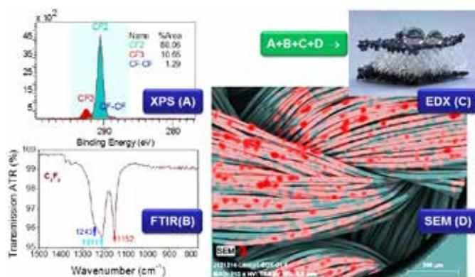
Correlated investigations (A+B+C+D) enable application-oriented optimisation of the properties of plasma-treated samples. The sample surface was coated with a fluorocarbon plasma polymer.
