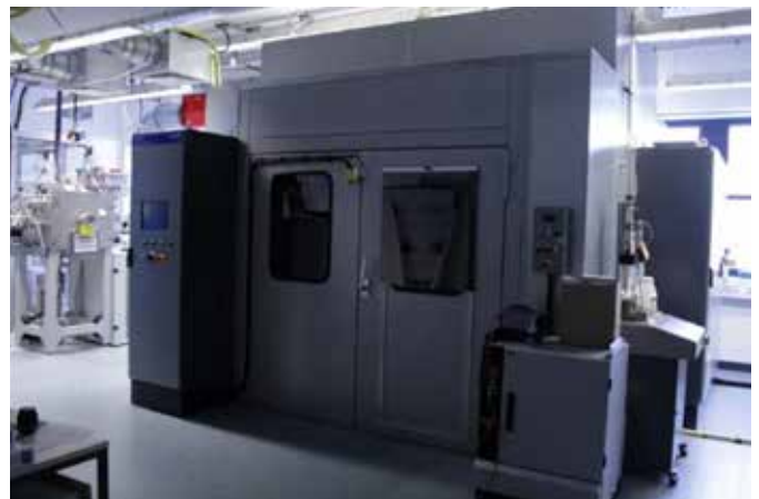
Industrial system for the thermal atmospheric pressure plasma spray process for producing functional films
