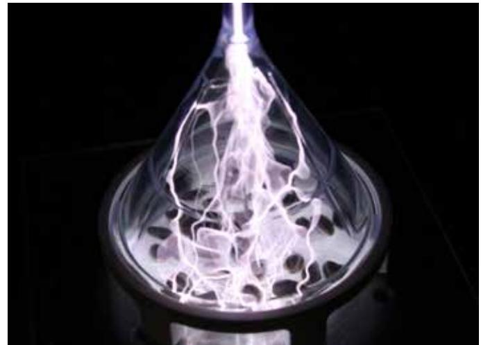
Treatment of sunflower seeds by corona discharge. The treatment kills micro-organisms on the surface of the grains. In addition, their ability to absorb water increases, and metabolic processes are stimulated.
