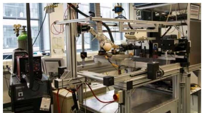
Set-up for carrying out welding tests with fixed torch position and moving work piece combined with equipment for imaging spectroscopy and high-speed kinematography.
