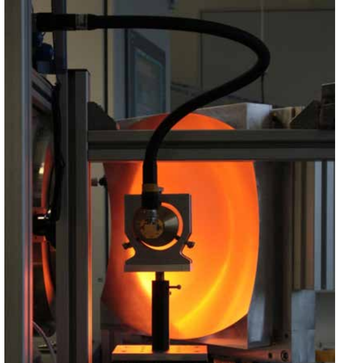
Electron density measurement with a 50 GHz interferometer at a low-pressure plasma discharge
