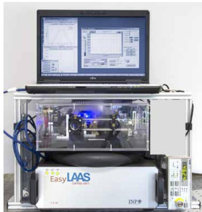
EasyLAAS system for laser absorption measurements
