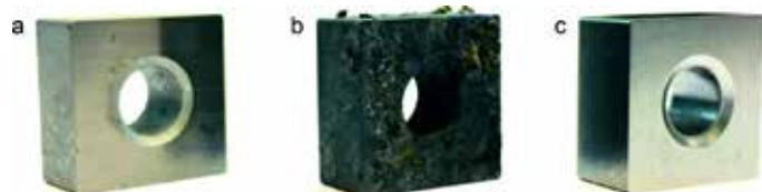
Test specimens in the PEP process: (a) untreated, (b) contaminated, (c) cleaned and polished
