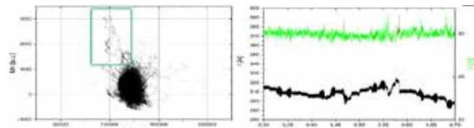
Green rectangle: Increased manganese output during a welding process. The same time is marked on the right side of the electrical signals. This deviation can be clearly detected only in the sensor signal.
