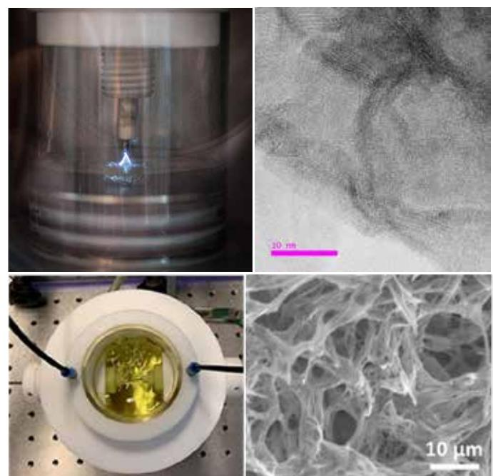
Figure: PiL process in tip-to-plate and tip-to-tip configuration for the synthesis of few-layer graphene and V<sub>2</sub>O<sub>5</sub> nanofibres
