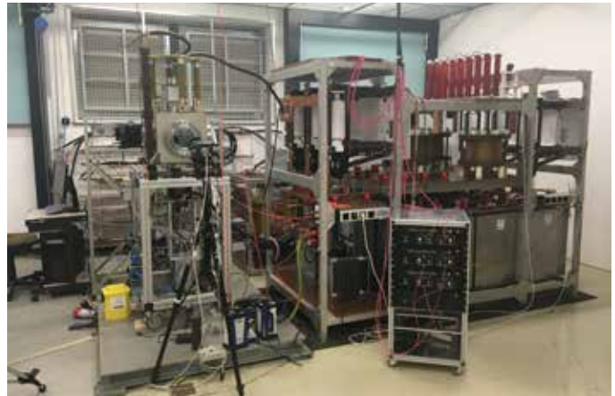
A view into the arc laboratory: Synthetic test circuit (right in picture, the INP's own development), vacuum chamber with pump system and drive (left in picture).
