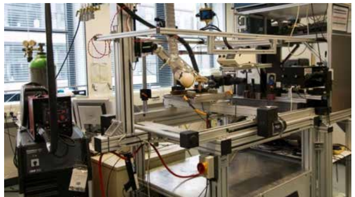
Set-up for carrying out welding tests with fixed torch position and moving work piece combined with equipment for imaging spectroscopy and high-speed cinematography.
