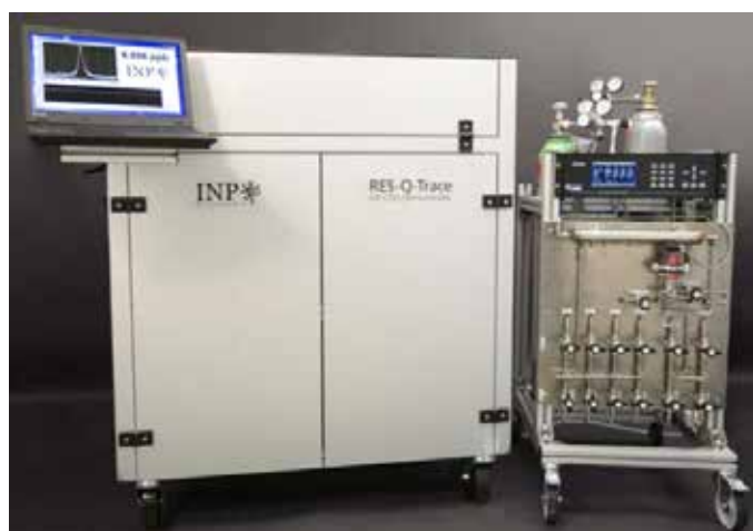
RES-Q-Trace – demonstrator of a resonator-based, quantum cascade laser-based trace gas analyser for highly sensitive trace gas detection.
