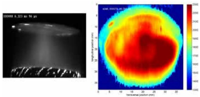
Snapshot of a vacuum arc (left) and temperature distribution of the upper electrode (anode) at 10 kA (right).
