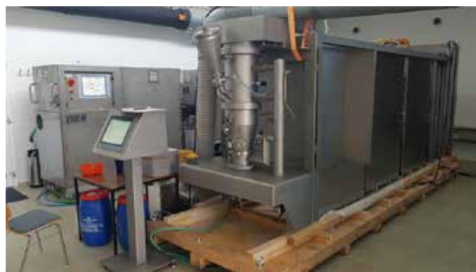
Fluid bed dryer with plasma gas generators (ADU)
