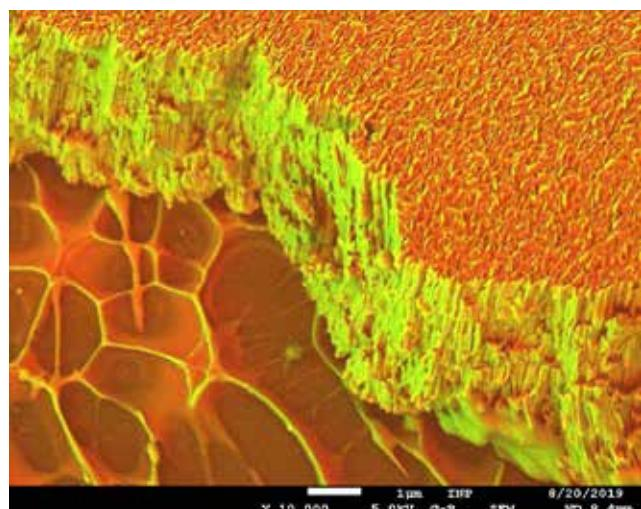
Electron microscopic image of the edge of a metal film (approx. 2.5  $\mu\text{m}$ ) produced at the INP for laser ablation (cooperation with the MPI für Plasmaphysik)
