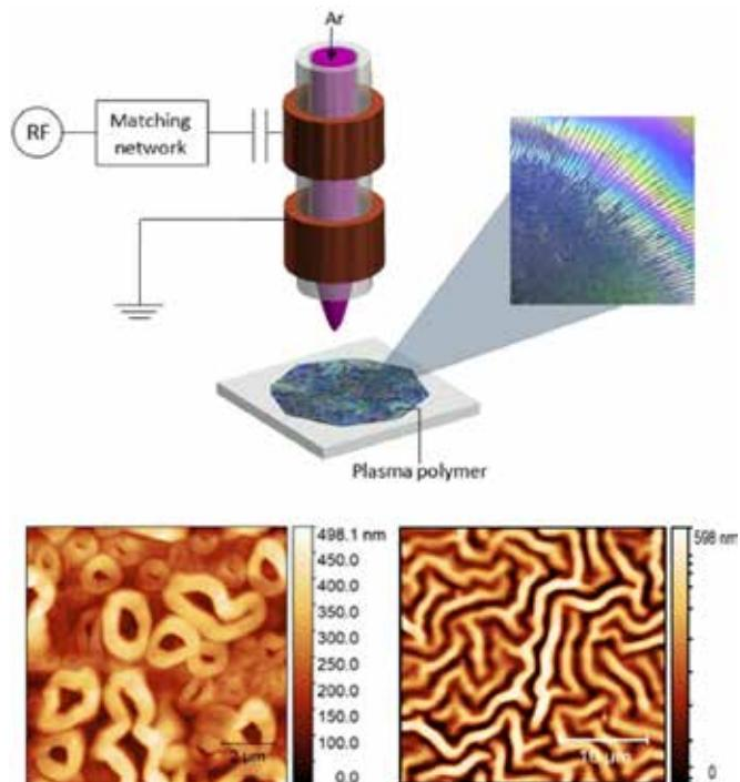
Schematic representation of the experimental set-up for the generation of functional coatings and hydrogels.
