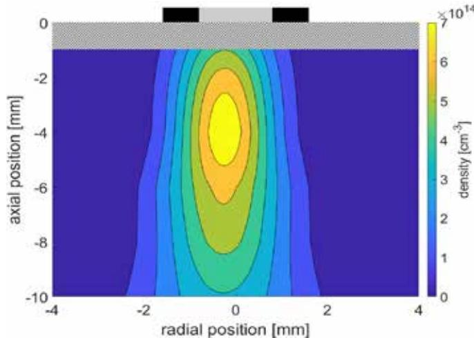
Profile of the distribution of the radical  $\text{HO}_2$  in the effluent of a plasma jet
