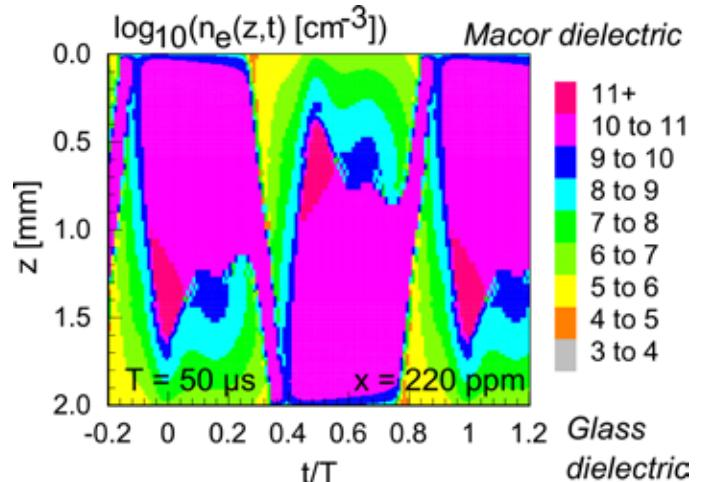
Spatio-temporal development of the electron density in a large-area dielectric barrier Ar discharge with the addition of  $x = 220$  ppm hexamethyldisiloxane for the deposition of silicon-organic films
