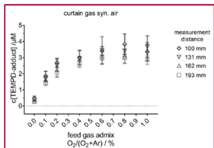
Electron spin measurement of ozone in physiological fluids. Depending on the admixture of oxygen to the working gas and independent of the distance ( $> 100$  mm), the TEMP signal increases significantly. The presence of ozone under these conditions was confirmed by measurements using a specific dye.
