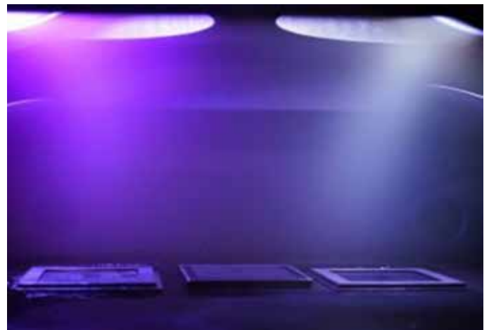
Production of a nanocomposite film using the PVD process
