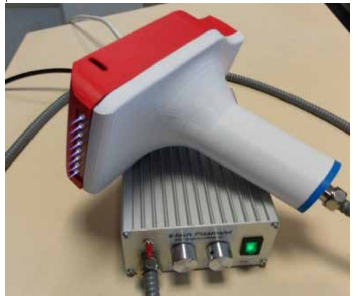
Laboratory sample of a plasma jet array for medical application based on the kINPen MED® for the treatment of larger areas
