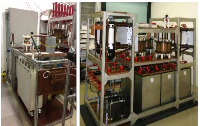
The newly constructed “Dora” overshoot voltage generator (left) and “Caesar” high-current generator (right) in the Institute’s arc laboratory
