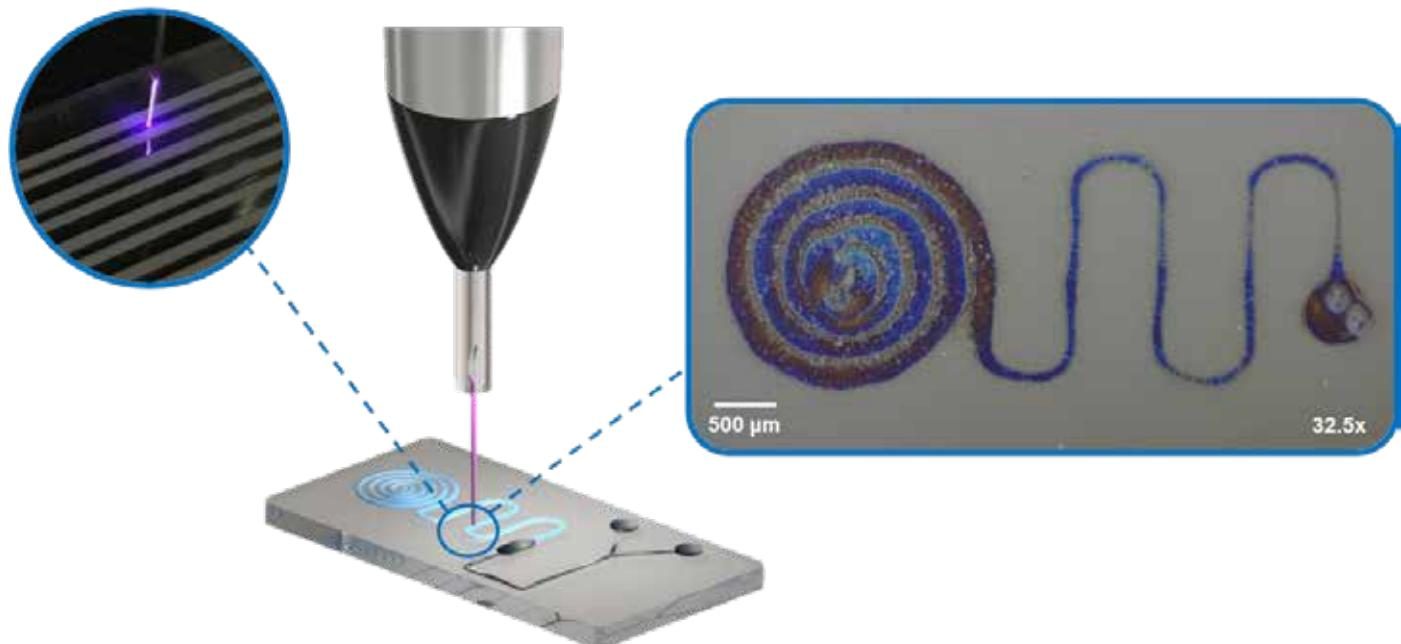
Schematic representation of the SurfAP3® plasma printer for the structured generation of functional layers and hydrogels with photographic images of the plasma discharge on an open microfluidic channel and a chemical structure generated with SurfAP3® on a silicon wafer.
