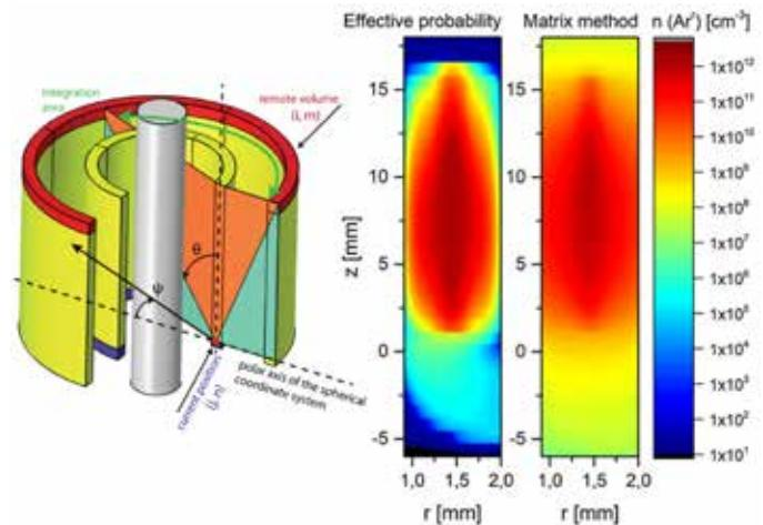
Results of modelling a non-thermal plasma jet in argon at atmospheric pressure from S. Valin et al., *Plasma Sources Sci. Technol.* 30 (2021) 115001. The geometric dependence of the volume element and non-local radiation contributions in the plasma jet (left) as well as a comparison of the density of the resonance atoms with approximation of the radiation transport by effective lifetime (middle) and with calculation by matrix method (right) are shown.
