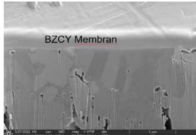
Proton conducting electroceramic thin-film membrane
