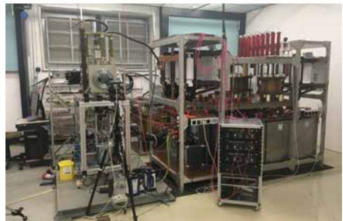
A view into the arc laboratory: Synthetic test circuit (right in picture, the in-house development of the INP), vacuum chamber with pump system and drive (left in picture).
