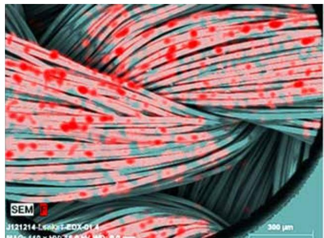
Electron microscope image of a textile fabric. Superimposed is the signal from the chemical analysis using energy dispersive X-ray analysis (EDX). Shown in red pseudocolour are traces of silicon-containing aggregates that were deposited in the textile during plasma treatment.
