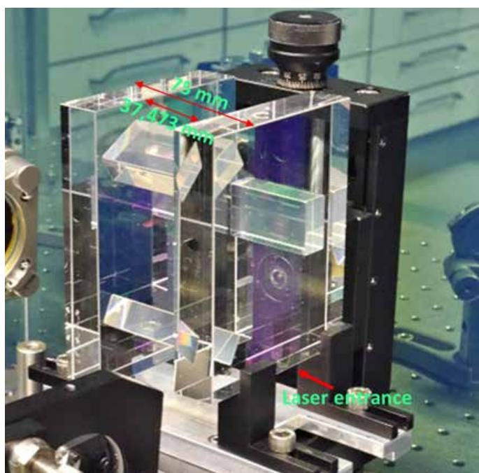
Photo of an air-spaced VIPA with laser coupling in the lower part of the coupling window
