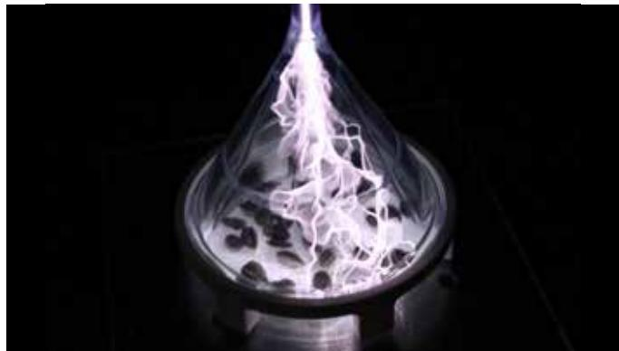
Small-scale seed treatment using corona discharge (funnel plasma source)
