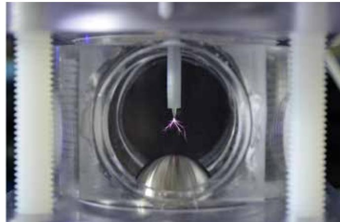
Representation of a discharge in water between a needle and a hemispherical electrode. It was generated with a 100 ns voltage pulse with an amplitude of approx. 60 kV.
