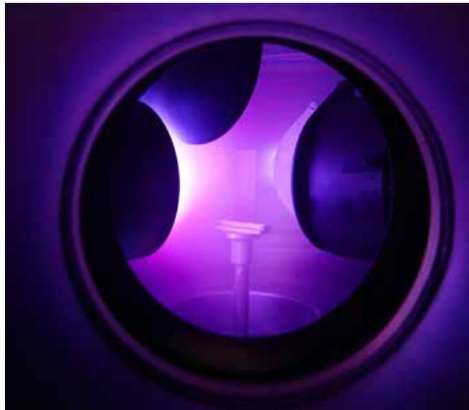
Coating method: Production of ceramic coatings using the PVD process: In the reactor, three starting materials can be evaporated simultaneously by cathode sputtering (magnetron sputtering).
