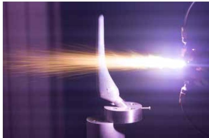
Thermal atmospheric pressure plasma spray process for the production of functional coatings. Shown here: Oxide layer on metallic implant
