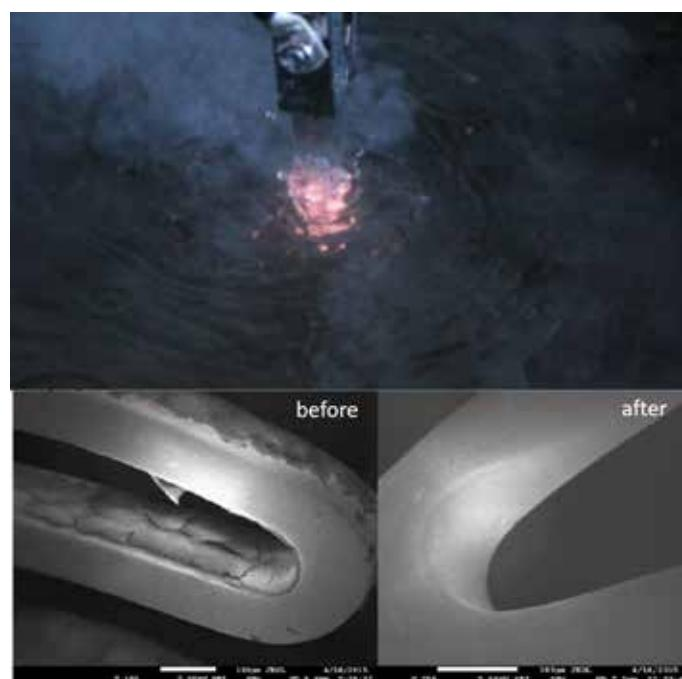
Plasma electrolytic polishing in use as fine cleaning and deburring for medical devices
