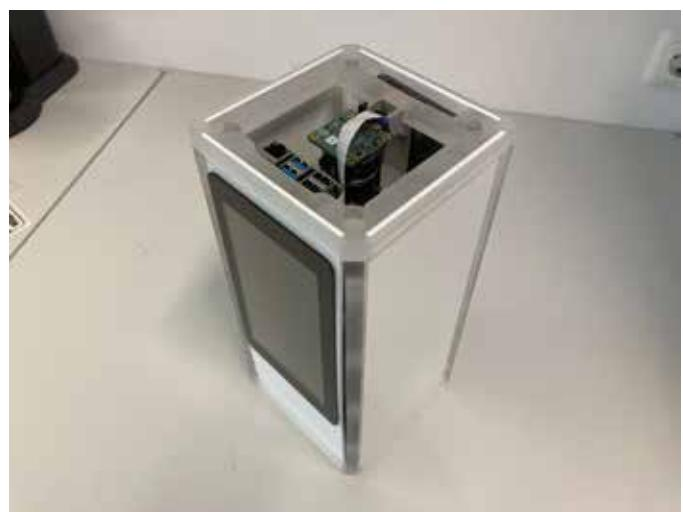
Camera-based material recognition system. The top cover has been removed in order to reveal the camera.
