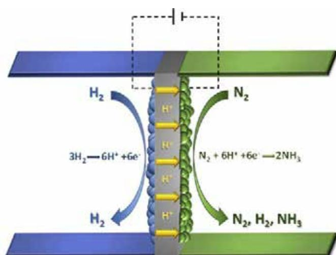
Schematic of a membrane electrode unit for the solid-state synthesis of ammonia.
