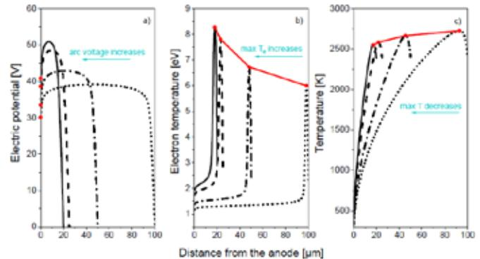
Results of the modelling of a thermal micro-arc within the DFG project "Theoretical description and modelling of arcs at small currents and small electrode distances" (Project number 390828847). The spatial variation of the electric potential (left), the electron temperature (centre), and the gas temperature (right) with variation of the electrode distance and a current density of  $10^6$  A/m<sup>2</sup> is shown.
