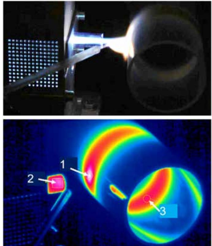
Microwave plasma for the synthesis of quartz glass for high-performance glass fibres. The layer is formed on a rotating glass cylinder. Above: Plasma jet source with effluent and supply of the reactive gas, Below: Measurement of the surface temperature (1: Outer wall 3: Inner wall of the cylinder, 2: Nozzle of the plasma source) during the process by means of an IR camera. "PLASFASTER" project, Leibniz competition (Baeva et al., J. Phys. D: Appl. Phys. 54 (2021) 355205).
