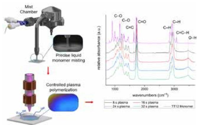
Schematic representation of part of the automated process for producing plasma-polymerised thin films at atmospheric pressure. The FTIR spectra of an acrylate-based monomer used and the corresponding plasma-polymerised films obtained at different polymerisation times show that the process allows the adjustment of the cross-linked polymer chains.
