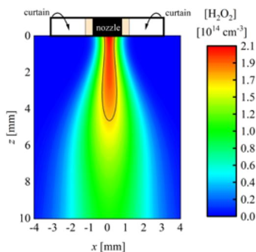
A contour plot of the  $\text{H}_2\text{O}_2$  particle densities in the effluent of the KINPen-sci
