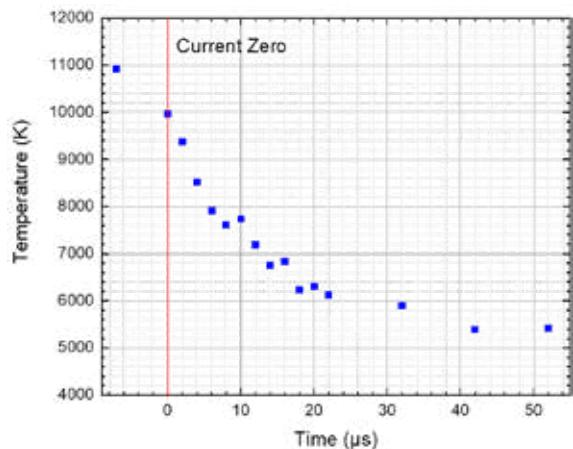
Development of the plasma temperature over time during and after the current phase (post-arc) of a hybrid switched-off DC switching arc (70A, 400 V DC)
