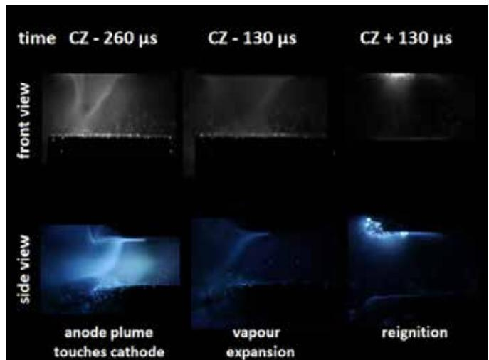
Snapshots of a vacuum arc around the current zero crossing (CZ) during thermal re-ignition as a result of strong electrode material evaporation. Current 10 kA.
