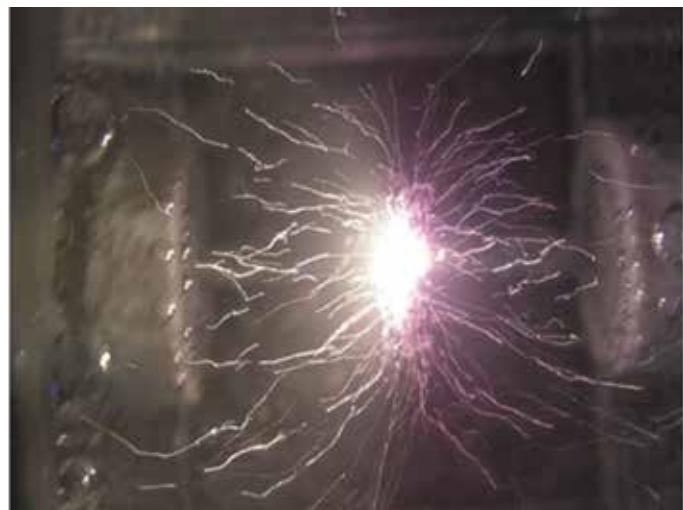
Electrical discharge in liquids: Synthesis of vanadium oxide/graphene nanohybrids as innovative battery materials
