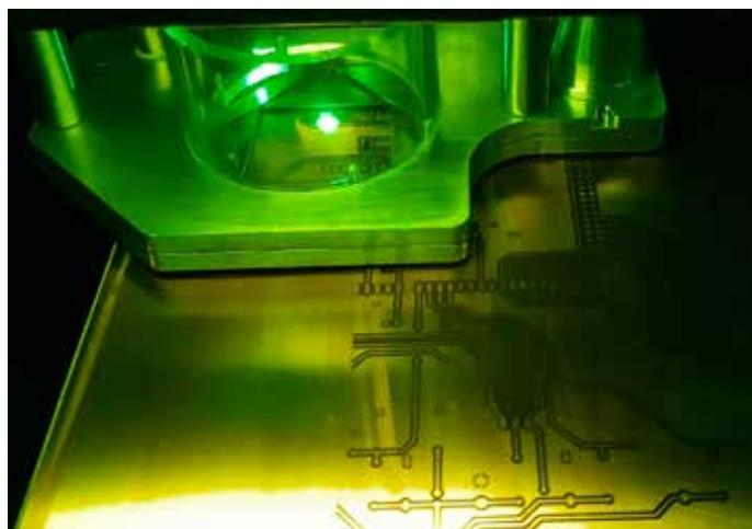
The solder side of a PCB is precisely structured in a laser process.
