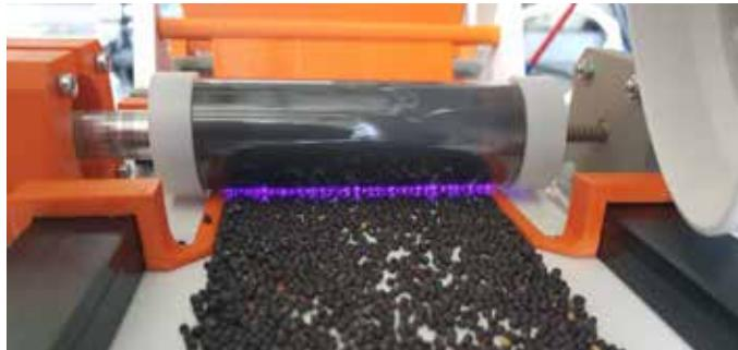
Continuous treatment of rapeseed by means of dielectric barrier discharge (conveyor belt plasma source)
