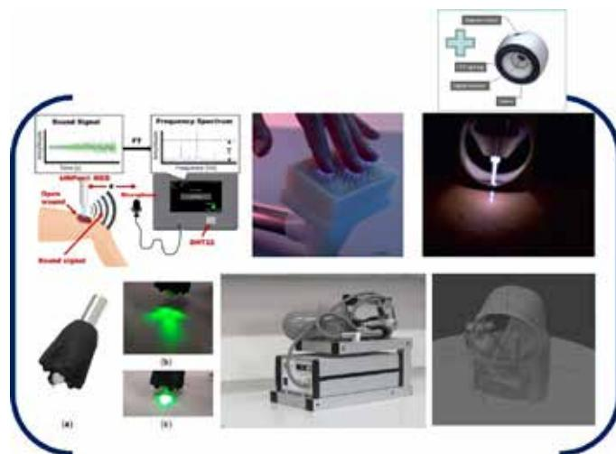
Device concept in the Ambuplas project – combination of acoustic operating time detection, visualisation of the effective area, and compatibility with different plasma sources
