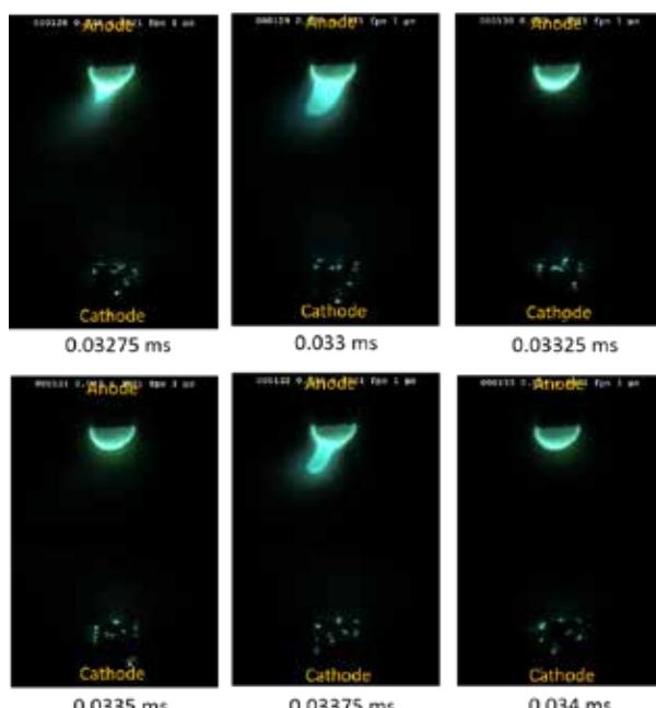
High-speed images of the observed oscillations of the anode plasma cloud of a high-current arc in vacuum
