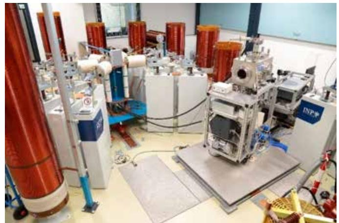
High-current generator for simulating various current courses in the electrotechnical field: AC pulses up to 200 Hz and 15 kA amplitude, AC pulses up to 80 kA at 50 Hz, DC pulses up to 20 ms duration and 10 kA amplitude and lightning impulse currents 10/350 $\mu$ s up to 50 kA max.
