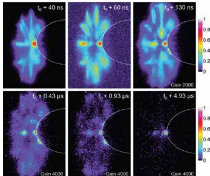
Formation of a discharge filament on a glass surface with a grid electrode in air behind it (expansion of approx. 5 mm).
