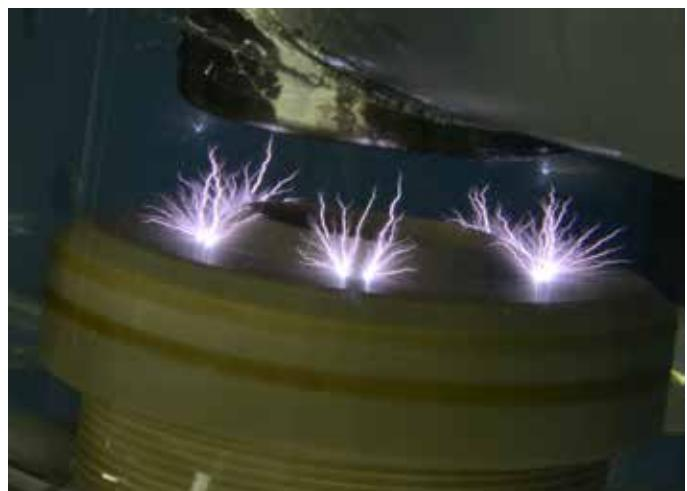
Spark discharge in water for biomass treatment
