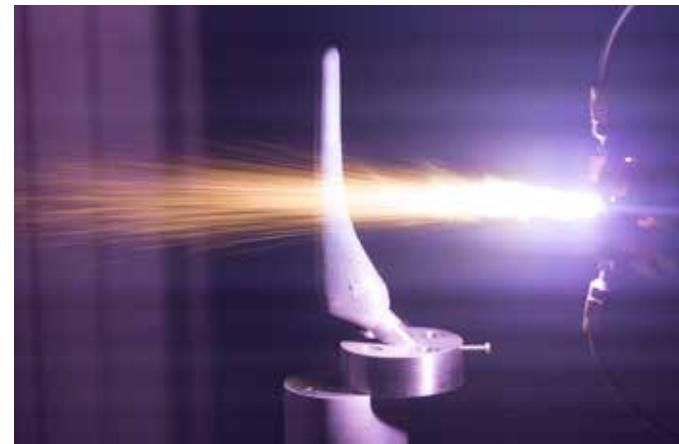
Thermal atmospheric pressure plasma spray process for the production of functional layers. Shown here: Oxide layer on metallic implant
