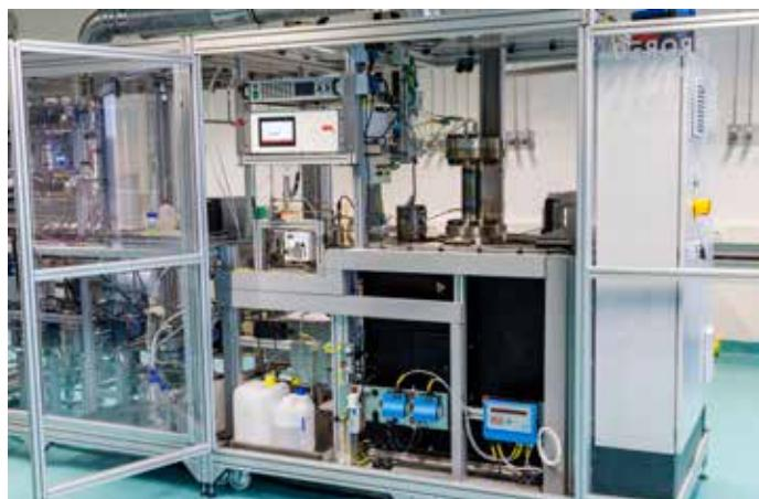
High-pressure test stand for the characterisation of tubular membrane-electrode units based on a sputtered proton-conducting perovskite membrane for use in solid-state ammonia synthesis.
