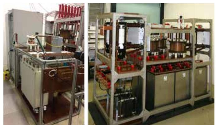
Left: Transient voltage generator (TRV) up to 45 kV @ 1 kHz. Right: High current generator (Weil-Dobke synthetic circuit type) up to 80 kA @ 50 Hz
