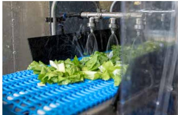
Plasma-treated water for the sanitation of fresh-cut lettuce in a commercially available washing machine. Microbial loads could be significantly reduced and this way a safer product for consumers is provided. Market introduction is pending approval of the method.
