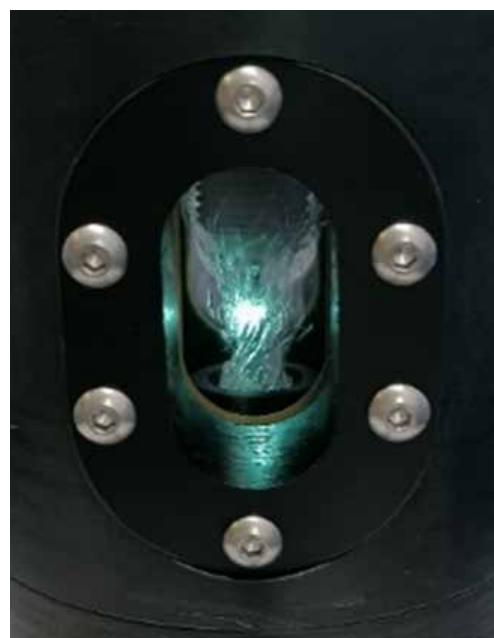
Sputter coating of a tubular substrate with a proton-conducting electroceramic thin film
