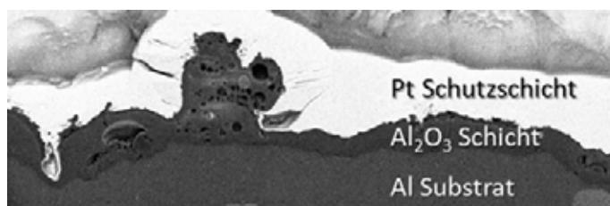
Top: Crystallographic analyses in the Bruker D8 Advance X-ray diffractometer. Bottom: Scanning electron micrographs of a PEO aluminium oxide layer in the FIB cross section
