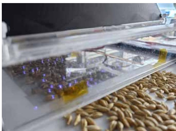
System for uniform treatment of seed with atmospheric pressure plasma at high throughput.
