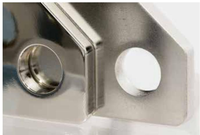
Plasma-electrolytic polishing: Comparison of a polished (left) and an unpolished component (right)
