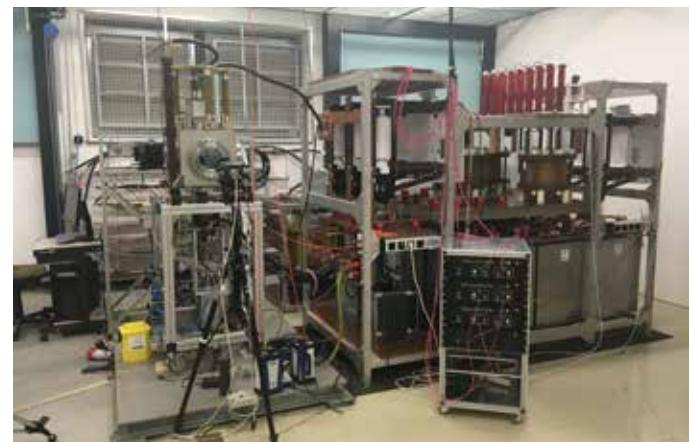
A view at the arc laboratory: synthetic test circuit (right in the picture, developed in-house by the INP), vacuum chamber with pump system and drive (left in the picture).
