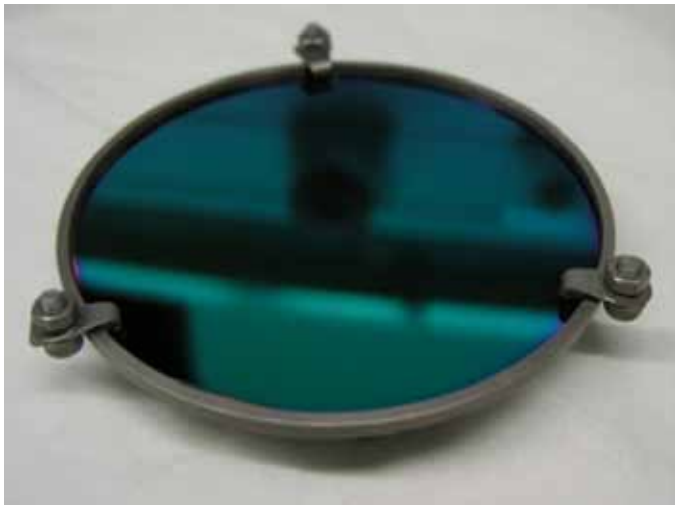
TiO 2 film on Si wafer produced by the PIAD process for measurement purposes
