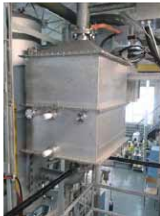
Stack reactor for test bench trials (left); installation of bypass in a marine diesel engine (right)
