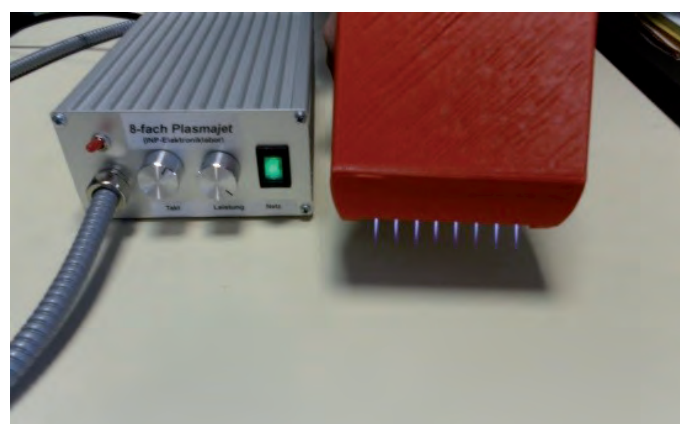
Fig. Laboratory prototype of a multi-jet with eight parallel plasma effluents
