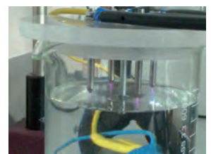
Fig. Experimental setup to for plasma activation of larger liquid volumes (max. 500 ml)
