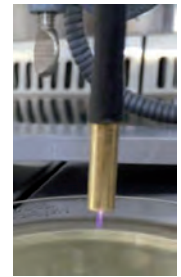
Fig. Laboratory prototype of a flexible plasma source for potential endoscopic application based on kINPen-technology
