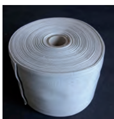
Fig 2: A „spool“ of the plasma source indicating the possibility of a roll-to-roll production.
