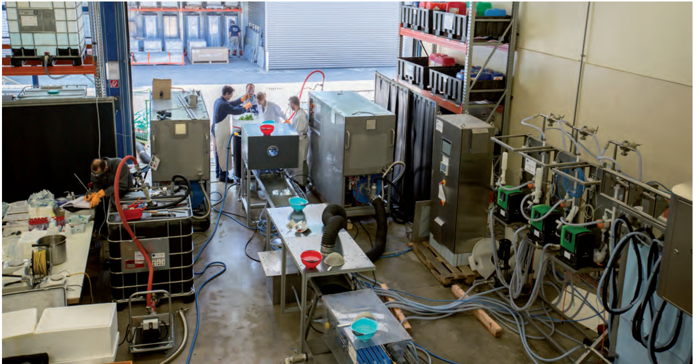
Figure 3: Technical center of Jürgen Löhre GmbH, Lübeck. Installation of the pilot plant with two INP plasma devices.
