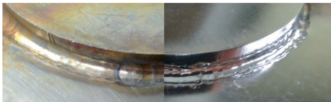
Fig. 2: Comparison between untreated stainless steel direct after processing without any cleaning (left) and after electrolytic plasma polishing (right).
