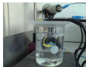
Fig. Experimental setup to for plasma activation of larger liquid volumes (max. 500 ml)
