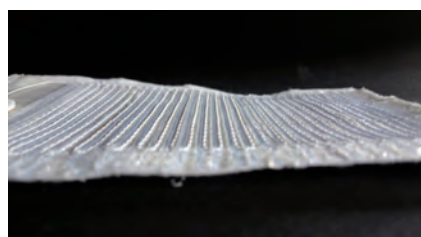
Fig 1: Side view of the plasma source showing the design of the electrodes.
