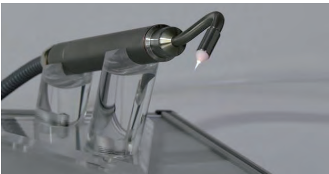
Fig. Laboratory prototype of a kINPen-based plasma device for intraoral application
