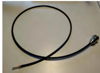
Fig. Laboratory prototype of a flexible plasma source for potential endoscopic application based on kINPen-technology
